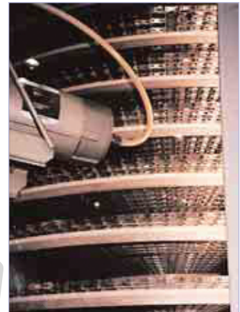
TIVAR® H.O.T. J-leg wearstrips are used in proofing ovens or food dehydrators.
