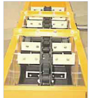
Grain drag flights manufactured from TIVAR® H.O.T. last longer and perform better in higher temperatures or where chemicals such as Hexane are used than those manufactured from standard UHMW.
